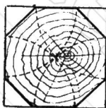
Fig. 7.—Octagon-section Blind Roller cut from Square-section Wood.
