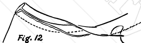
Figure 12 —To make a bias facing, cut and join 1\frac{1}{4} " bias strips as in figures 7 and 8, page 21. Stitch strip to edge, right sides together, mitering corners. Trim seam to \frac{1}{8} ". Turn strip to wrong side, turn under raw edge and slip stitch (see figure 4, page 21) to inside of cap.
