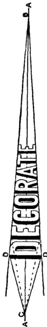
Fig. 135.—Simple Method of Drawing Letters in Perspective.
