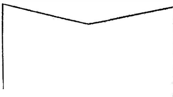
Fig. 24. If the line at the top of the apron pattern is straight, the material will V at the center front when cut
